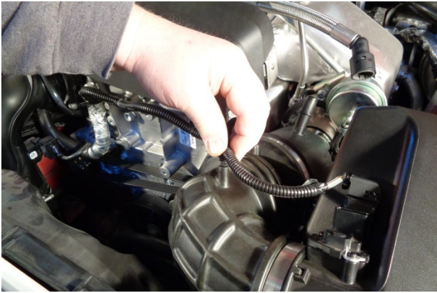
6. Release the MAF sensor lead clamp from the intake duct.
