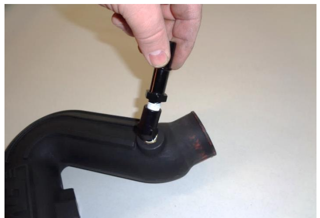
17. Apply 2 wraps of nylon thread tape to threads of 5/8" quick disconnect union (17), and install union in elbow.
