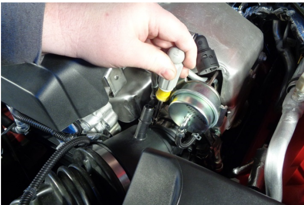
7. Loosen the hose clamp securing the intake duct to the turbine inlet.
