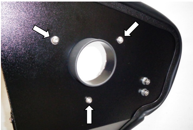
13. Attach air filter adapter (3) to heat shield using M6 screws (12), lock washers (11) and flat washers (10).
