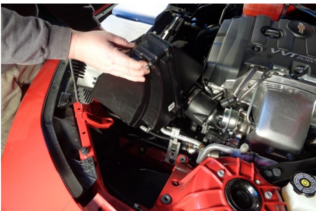
8. Grasp each corner of the airbox, one at a time, and firmly pull straight up to release each mount pin from its rubber grommet. After releasing all three pins, remove the assembled airbox and duct from the vehicle.
