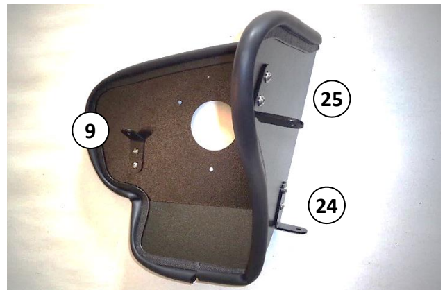
11. Attach brackets to heat shield (13) at the locations shown, using ¼-20 screws (7) (on the bracket side), and flat washers (4), lock washers (5) and nuts (6) (on the heat shield side). NOTE: Orient tab on bracket (9) upward.
