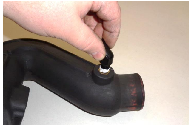
16. Apply 2 wraps of nylon thread tape to threads of elbow (16), and install elbow in intake tube (15).
