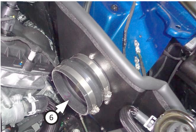
18. Place (x2) clamps (11) onto hump coupler (6) then press it onto airbox. Tighten clamp around adapter.
