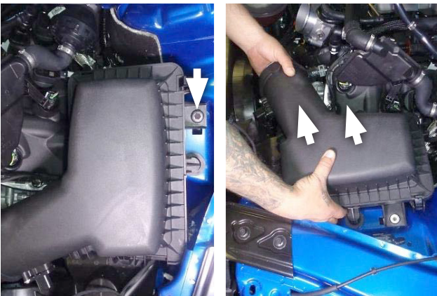
11. Remove and retain bolt securing airbox to vehicle frame then lift airbox straight up to remove it from vehicle.
