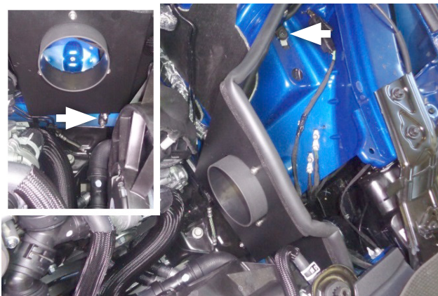
17. Install airbox into vehicle using factory bolt (removed step 12) on upper bracket, then use screw (24) , split lock washer (25) and flat washer (26) on lower bracket. Finally, fully tighten both brackets to airbox.
