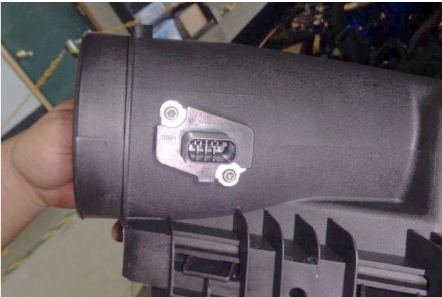
12. Remove MAF sensor from airbox then remove stock gasket from sensor.
