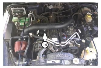
15. Apply PTFE tape to **male barb (14)** then install it into intake tube, oriented as shown.
