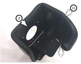
Starting at corner indicated, press airbox gasket
