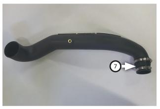
13. Place hose clamp (8) onto small end of rubber coupler (7) and hose clamp (9) onto larger remaining end of coupler. Place assembly onto intake tube as shown then tighten clamp.
