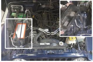
4. Unlatch and remove airbox cover, remove filter from airbox, then unbolt and remove airbox from vehicle.
