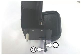
Insert screw (22) through bracket (5) and washer (18) then fasten assembly to airbox with flat washer (24), split lock washer (23) and nut (19).
