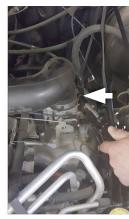
Loosen clamps at both ends of intake then remove it from vehicle.
