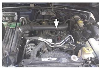
2. Open hood then disconnect PCV hose from tube and remove it.
