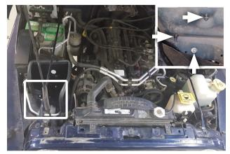
8. Set airbox into engine compartment, matching screws with holes in body. Reach through wheel well and fasten airbox with (x3 ea.) flat washers (24), split lock washers (23) and nuts (19).
