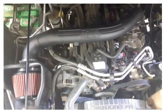
14. Place intake assembly onto throttle body and adapter in engine compartment. Press couplers against stops then center tube. Tighten screw clamps completely.
