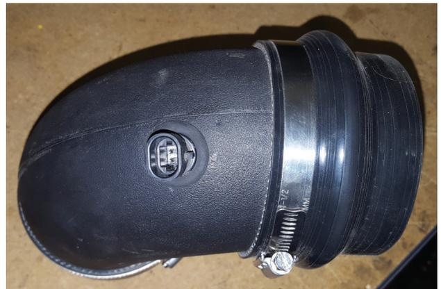
3. Install IAT sensor (removed step 1) in through grommet and tube. Use soapy water to ease insertion if necessary.
