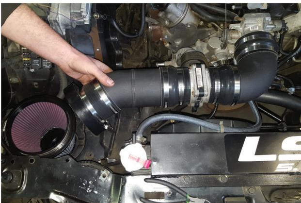
3. Install air filter adapter onto air intake assembly.
