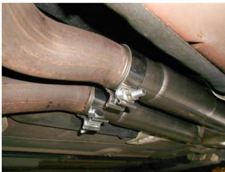
1) Begin the installation by placing a supplied 2-1/2" clamp onto each of the inlets of the X-pipe assembly **#26552M**. Then, place the X-pipe onto the back of the stock head pipes (the embossed Hurst H will be facing the ground). Level and center the assembly in the drive line tunnel and support with a stand. Tighten the two clamps enough to hold, but still allow for adjustment.
