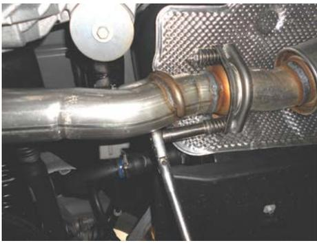
2) Using a 13mm socket, unbolt the left tailpipe assembly at the flanged connection at the rear of the muffler. Slide the three hanger rods out of the rubber mounts on the vehicle and remove the left tailpipe assembly.
