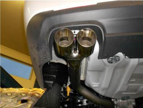
3) Place a supplied clamp onto the left muffler outlet. Place the left tailpipe **#26556M** into position and starting from the rear, connect the hangers on the tailpipe to the rubber mounts on the vehicle. Slide the tailpipe fully into the muffler outlet. Adjust the tailpipe so that the stainless tip is level and centered in the bumper cut-out. Tighten clamp enough to hold, but still allow for adjustment. Repeat this step for right tailpipe **#26557M**.
