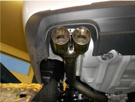
7) Place a supplied clamp onto the left muffler outlet. Place the left tailpipe **#26580M** into position and starting from the rear, connect the hangers on the tailpipe to the rubber mounts on the vehicle. Slide the tailpipe fully into the muffler outlet. Adjust the tailpipe so that the stainless tip is level and centered in the bumper cut-out. Tighten clamp enough to hold, but still allow for adjustment. Repeat this step for right tailpipe **#26581M**.
