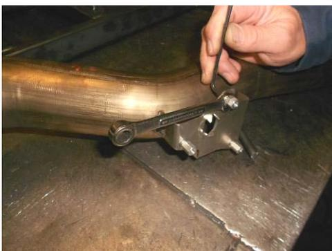
2) Mount with the spacers and washers, attached. Tighten securely.
