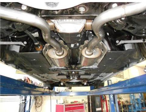
4) Adjust the position of the pipes, mufflers and tips to provide a satisfactory fit. A minimum of 1/2" clearance around all parts of the system must be maintained; while keeping suspension travel and vibration in mind. After adjustments have been made, you may now securely tighten all clamps. Check for adequate clearance between the X-pipe and body braces.
