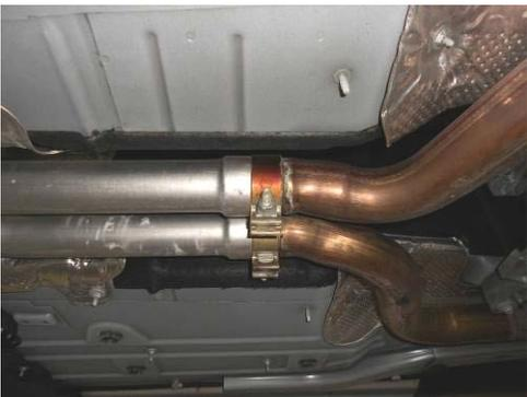
4) Support the right side of the system with a stand, then using a 15mm socket, loosen the clamps at the slip fit connections behind the catalytic converters. Unclip the grounding strap from the middle hanger on the right side of the vehicle. Remove the three remaining hanger rods from the rubber mounts on the vehicle, then carefully lower the stand at the rear of the vehicle and with the help of an assistant slide the system back off of the head pipes and lower the system from the vehicle.
