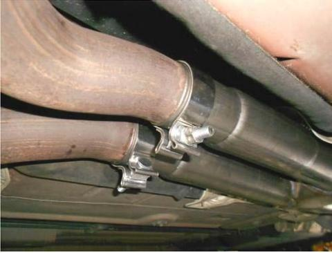
1) Begin the installation by placing a supplied 2-1/2" clamp onto each of the inlets of the X-pipe assembly **#86367M**. Then, place the X-pipe onto the back of the stock head pipes (the embossed Hurst H will be facing the ground). Level and center the assembly in the drive line tunnel and support with a stand. Tighten the two clamps enough to hold, but still allow for adjustment. Reinstall the two front body braces and tighten securely.
