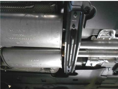
3) Using the same 13mm socket, unbolt the two body braces between the catalytic converters and the mufflers. Place the two braces and nuts aside for reinstallation after the Flowmaster system is installed
