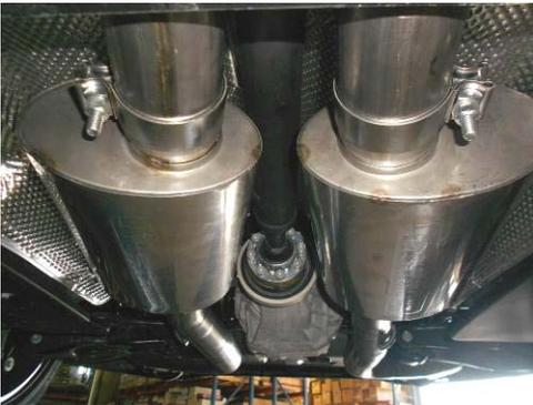
2) Place a supplied 2.50" clamp onto the inlet neck of both mufflers. Slide the mufflers onto the back of the Scavenger X-pipe assembly and support with stands. Level the mufflers and tighten the clamps enough to hold, but still allow for adjustment.
