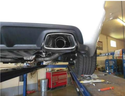
3) Place a supplied clamp onto the left muffler outlet. Place the left tailpipe **#86372M** into position and starting from the rear, connect the hangers on the tailpipe to the rubber mounts on the vehicle. Slide the tailpipe fully into the muffler outlet. Adjust the tailpipe so that the stainless tip is centered in the exhaust bezel. Tighten clamp enough to hold, but still allow for adjustment. Repeat this step for right tailpipe **#86371M**.
