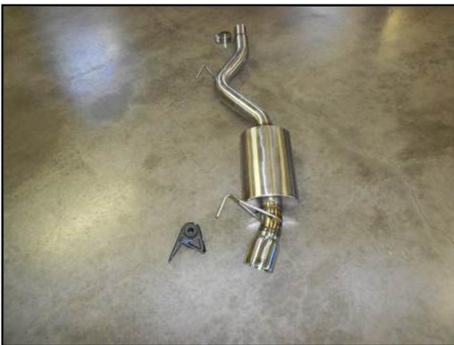
1) Place the new Hurst muffler units next to the factory units and swap the front and rear hanger mounts from the stock mufflers to the Hurst assemblies. Also, place a provided 2.25" clamp onto the inlet of each assembly. Tighten the clamp just enough to hold in place.
