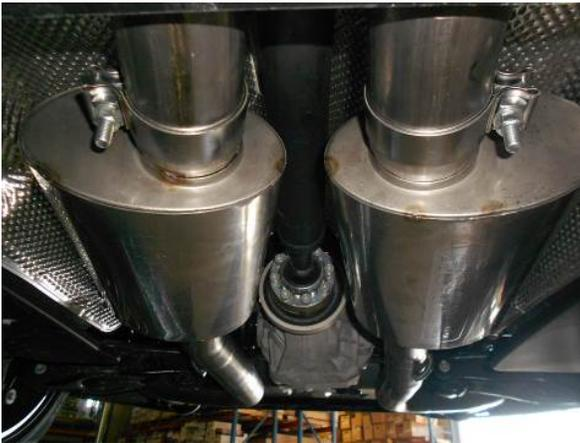
6) Place a supplied 3" clamp onto the inlet neck of both mufflers. Slide the mufflers onto the back of the Scavenger X-pipe assembly and support with stands. Level the mufflers and tighten the clamps enough to hold, but still allow for adjustment.
