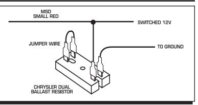
Figure 7 Wiring the Dual Ballast Resistor for Run-On.
