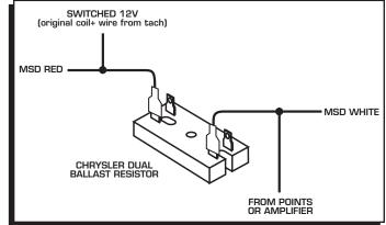
Figure 5 Wiring the Dual Ballast Resistor.
