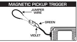
Figure 9 Checking for Spark with Magnetic Pickup.
