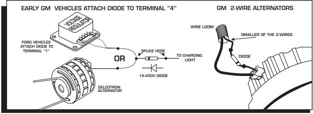
Figure 6 Installing the Diode to fix Run-On.
