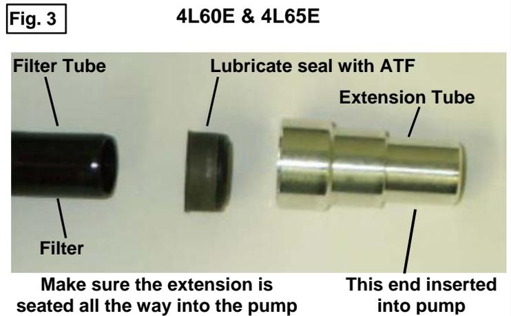
5. For the TH-700 R4 and 4L60 transmissions, install the supplied O-rings on the extension tube provided in the kit (See Figure 4). Lubricate the seal on the filter (B&M recommends that the filter be changed at this time) and the O-rings with transmission fluid. Place the extension tube on the oil filter. Install the assembly into the oil pump bore.
