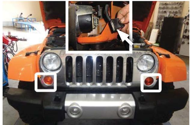
2. Unplug turn signals (x2) by sliding back tab, depressing lever and pulling out connector.
