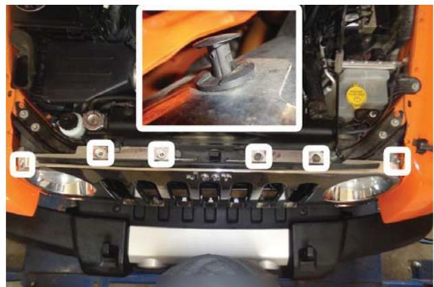
3. Remove push pins (x6) holding grill cover to vehicle frame. Retain pins for later use.
