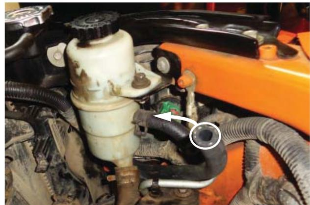
15. Route and trim transmission hose to length to reach power steering port without creating kinks or sharp bends in hose. Retain remaining hose. Do not disconnect factory hose at this time.
