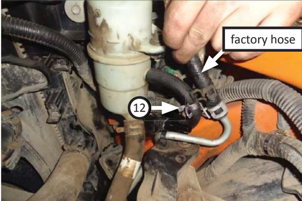
19. Place **pinch clamp (12)** onto transmission hose (from step 15). Pull and lift factory hose from PS port and replace it with transmission hose.
