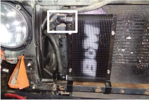
17. Seat transmission hose fully onto 45° barb then move pinch clamp into position over connection.
