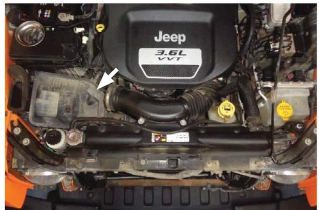
22. Re-install airbox base (removed step 6).
