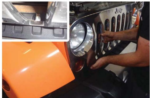
4. Pull straight out along bottom of grill cover to unclip it, then remove it completely from vehicle. Retain for later use.
