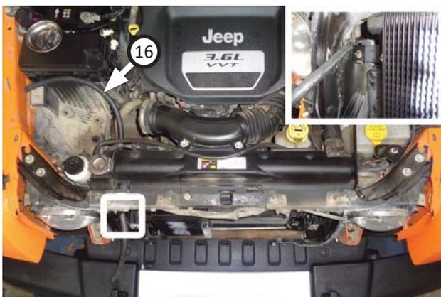
13. Feed  $\frac{3}{8}$ " transmission cooler hose (16) through corner of radiator frame into airbox holding space. If necessary, trim rubber airdam in top corner to make room for cooler hose.
