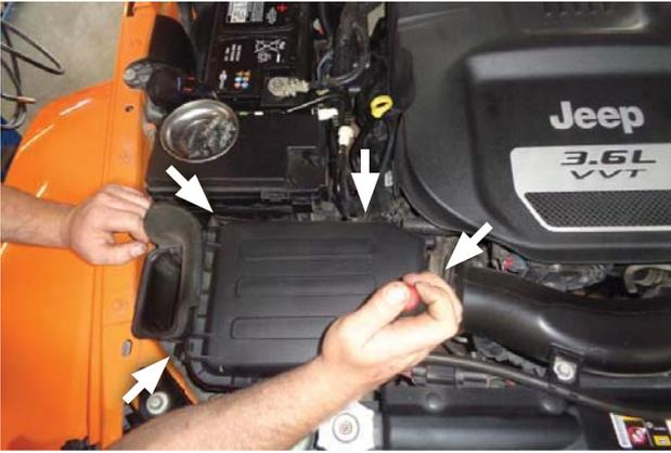
23. Re-install airbox cover (removed step 5) and secure it to base using latches. Tighten screw clamp holding resonator assembly to airbox.
