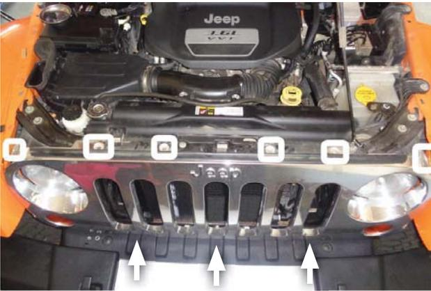
24. Place grill cover (removed step 4) back in place then push along lower section to clip it into position. Re-install push pins (x6) (removed step 3) along top of grill cover.
