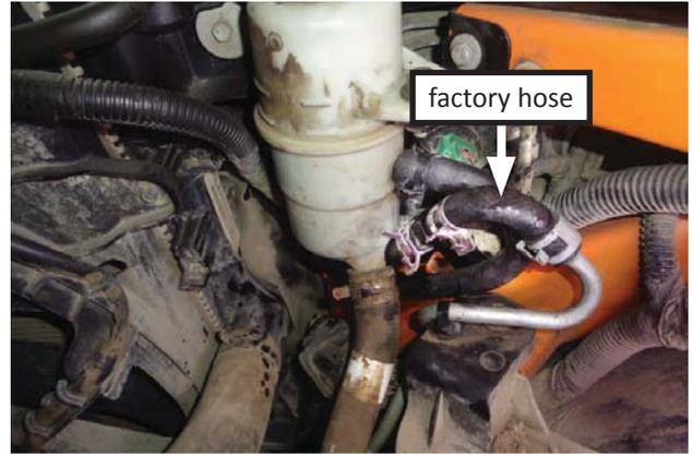
20. Connect factory hose to straight barb. Move pinch clamps (x2) into position over connections.
