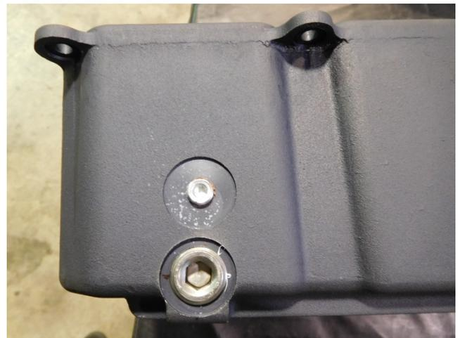
4. Locate the threaded boss inside of the transmission pan. Set the 2" magnet over the boss and secure it in place using the supplied M 6x10mm bolt and M6 lock washer.
