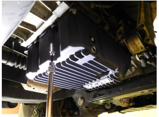
7. The new B&M transmission pan also includes a ¼ NPT port above the drain plug that can be used for an optional transmission temperature gauge. (available separately)
