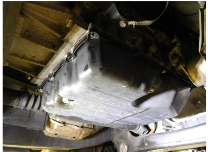
7. Remove old trans pan gasket and the “check” plug off the factory pan. We recommend you clean and thoroughly inspect the current condition of the gasket before reusing. Install pan gasket and factory “check” plug onto the B&M trans pan.
