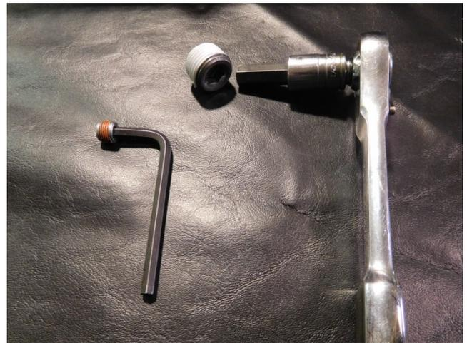
3. Install the drain plug and accessory port plug on the new B&M trans pan while you wait for the old trans fluid to drain.
