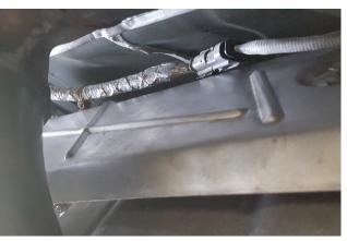
15. Allow exhaust to cool then re-install. Also install side cover and wire loom (removed step 4).
