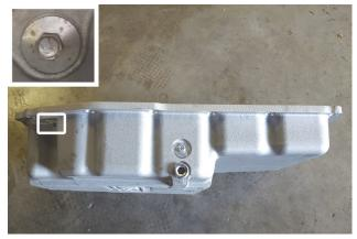
10. Make sure check bolt (removed step 3) still has seal, then install it into deep pan.
