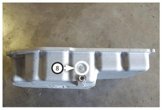
This kit includes a ½ NPT port above drain plug that can be used for an optional transmission temperature gauge. (available separately) Otherwise, install NPT plug (8).
