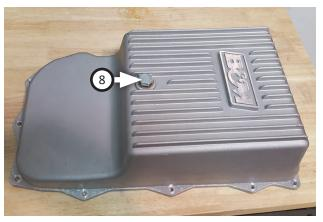
7. Fasten **plug bolt (8)** through **drain gasket (9)** into deep pan as shown.
