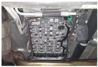
5. Remove (x13) factory bolts and pan from vehicle.
