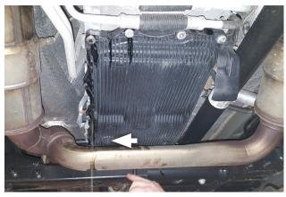
**NOTE:** To avoid fluid draining onto your exhaust pipes, use a funnel to direct it into your pan.
