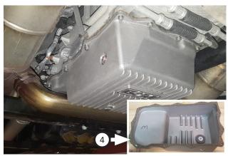
10. Set gasket (4) onto deep pan then set it into place on transmission, securing it with (x13 ea.) bolts (6) and flat washers (7). Torque screws to 8ft lbs.
