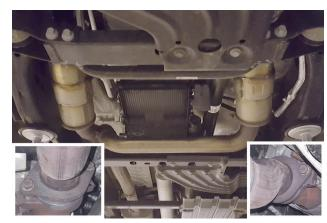
If you have limited access to your transmission pan, unbolt exhaust flanges from manifolds and lower exhaust system onto stands.
