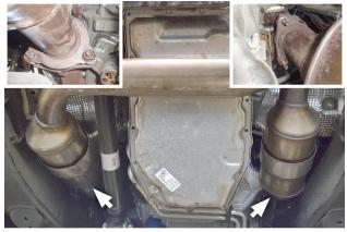
Remove (x3 ea.) nuts securing passenger and driver side exhaust manifolds to exhaust pipe. Then pull headers from their mounts.
