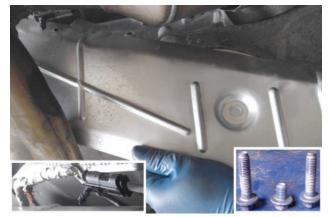
4. Remove wire loom, remove bolts (x3) and side cover from passenger side of transmission. Retain for later re-use.
