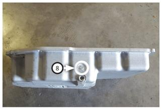
This kit includes a ¼ NPT port above drain plug that can be used for an optional transmission temperature gauge. (available separately) Otherwise, install NPT plug (8).
