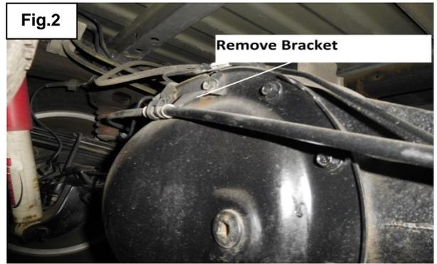
7. Now remove the lower tab from the emergency bracket to allow clearance once reinstalling back on the B&M diff cover. (See Figure 3)
