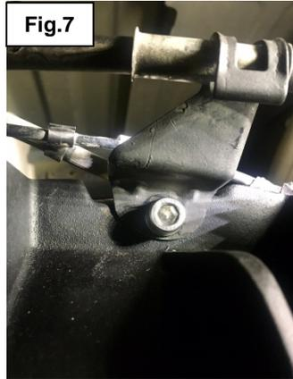
15. Install the rest of the supplied bolts and washers and torque to 15ft.lb in a crisscross pattern.
