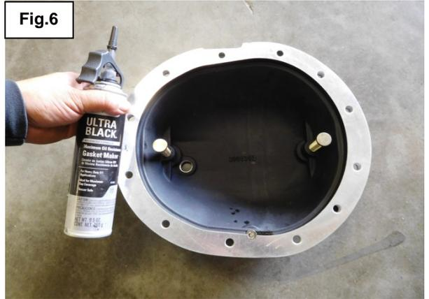
13. Install the B&M Cast Aluminum Rear End Cover on the axle housing using a supplied bolt and washer at a bottom hole on the cover so it can be used as a guide
