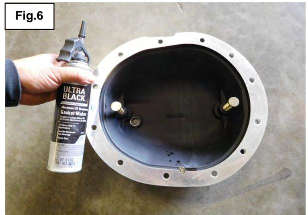
13. Install the differential cover on the axle housing using a supplied bolt and washer at a bottom hole on the cover so it can be used as a guide
