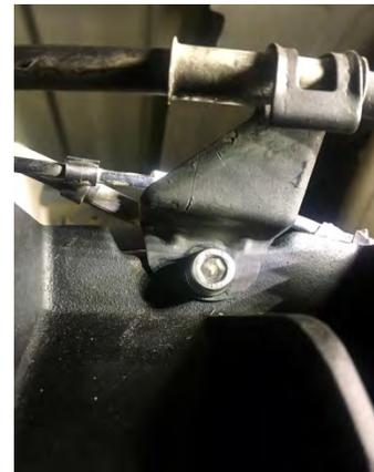
15. Install the rest of the supplied bolts and washers and torque to 15 ft-lbs in a crisscross pattern.
