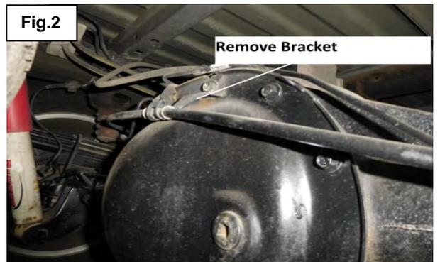
7. Now remove the lower tab from the emergency cable bracket to allow clearance once reinstalling back on the B&M diff cover.
