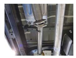
1) Connect the flange on inlet pipe assembly **#26668M** to the factory flange behind the flex pipe, then connect the hanger on the pipe to the rubber mount on the vehicle. Reinstall the two nuts and tighten enough to hold, but still allow for adjustment. Support the rear of the pipe with a stand.
