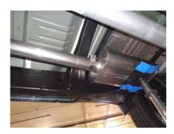
2) Place the provided 3" clamp over the inlet of the muffler, then slide the inlet of muffler onto the back of the inlet pipe. Use a stand to support the muffler. Tighten the clamp just enough to hold in position. Note: The protective plastic wrap has been left on the muffler to protect the finish, please remove prior to starting the vehicle.
