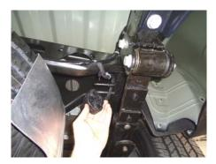
3) Place the provided 2 ¼" clamps onto the muffler outlets. Then remove the 3 factory rubber exhaust isolators from the mounts on the vehicle, two just forward of the rear axle and one at the rear of the vehicle.
