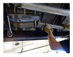
3) Using a 15mm wrench, loosen the two nuts on the flanged connection behind the catalytic converter. Retain the nuts, they will be re-used. Separate the hanger on the pipe from the rubber mount on the vehicle and lower the inlet pipe and muffler from the vehicle.
