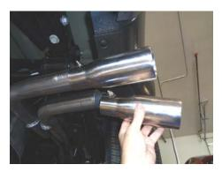
6) Place the **#ST439** stainless tips onto the ends of the tailpipe assembly and adjust to the desired position. Tighten the pinch clamps on the tips enough to hold in position.
