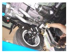
5) Place tailpipe assembly **#86441M** into position over the rear axle and slide into the muffler outlets. Support the rear of the assembly with a stand and connect the rubber hangers on the assembly to the wire mounts on the vehicle. Be sure that the pipes are fully seated in the muffler and tighten the clamps enough to hold in position.
