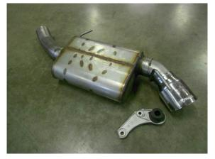
1) Place the new Flowmaster muffler units next to the factory unit and swap the rear hanger mounts from the stock muffler to the Flowmaster assemblies. **Note:** The protective plastic wrap has been left on the mufflers to protect their finish, please remove prior to starting the vehicle.
