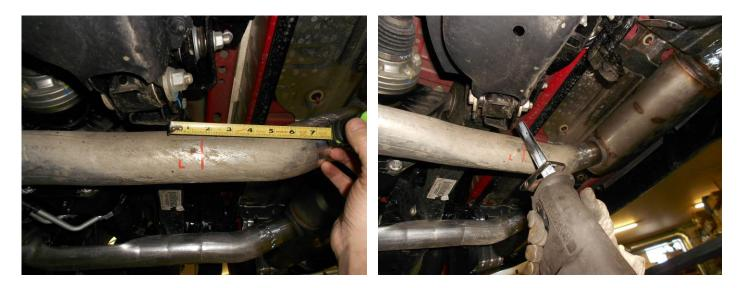
2) Begin by measuring back 1 ½" from the rear of the suspension cross-member shown in the photos above and make a mark on both pipes. Support the exhaust system both in front and behind the area to be cut, then once you've double checked that the measurements are correct, cut both pipes at the marks. **Note: Use caution when cutting!**
