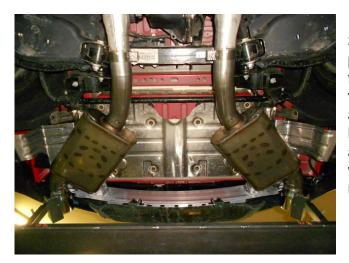
3) Adjust and level the two muffler assemblies to provide a satisfactory fit. They can also be adjusted forward or back to get the desired position in the rear valance cut-outs. A minimum of 1/2" clearance around all parts of the system must be maintained; while keeping suspension travel and vibration in mind. After adjustments have been made, and you are satisfied with the fit, you may now securely tighten the two muffler inlet clamps.
