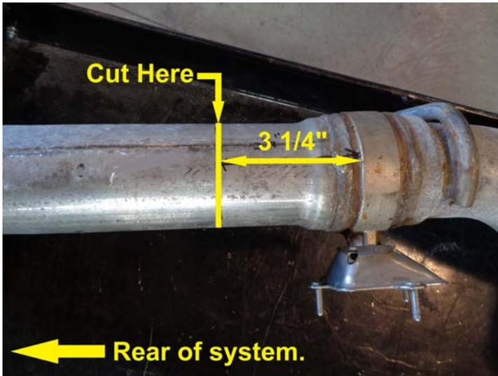
On the passenger side of the system, Measure back 3 1/4" from the cast body of the exhaust valve and make a mark. Using a hacksaw or sawsall, cut the pipe through on this mark. After cutting, remove any burrs from the end of the pipe using a file or die grinder.
