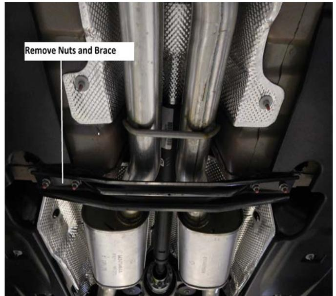
3) Place a stand under the rear of each tailpipe to support the rear of the system. Just forward of the rear differential, you will find two exhaust valve actuators, one mounted to the side of each tailpipe. Carefully unplug the wire from the actuator and tuck away for reconnection later.
