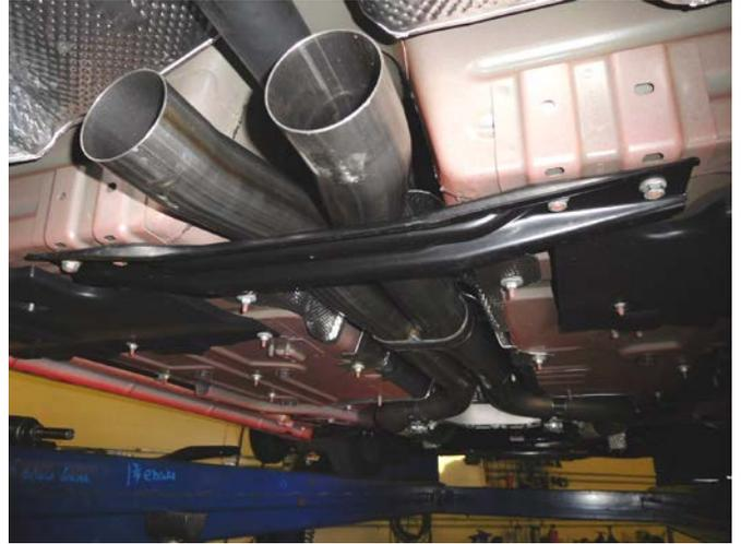
2) Place a supplied 3" clamp onto the inlet neck of both mufflers. Slide the mufflers onto the back of the Scavenger pipe assembly about 1-3/4" and support with stands. Level the mufflers and tighten the clamps enough to hold, but still allow for adjustment.
