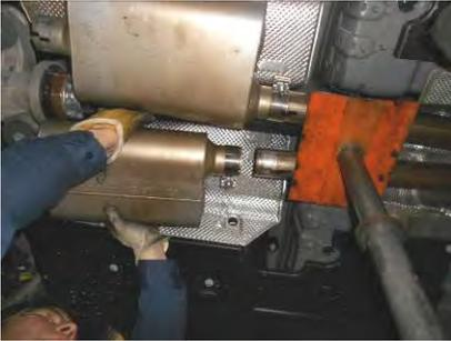
3) Place a supplied 2 ½” clamp onto the inlet of each **#71226-Z** muffler. Then fully slide the mufflers onto the back of the Scavenger pipe assembly and support with stands. Level the mufflers and tighten the clamps enough to hold, but still allow for adjustment.
