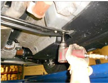
2) Using a 13mm socket, unbolt the two body braces in the center of the vehicle and set aside. The braces will be re-installed after completing step 2 of the installation instructions below.
