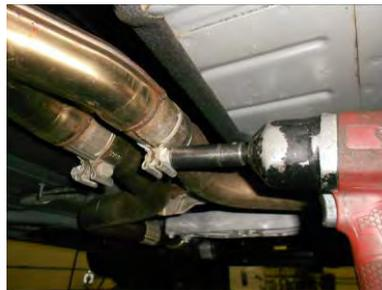
4) Support the rear of the system with a stand, then starting at the rear of the vehicle remove the three hangers on the right side of the system from the rubber mounts on the vehicle. Unclip the ground strap from the middle hanger on the right tailpipe and using a 15mm socket, loosen the clamps at the slip fit connections behind the catalytic converters. Then with the help of an assistant, lower the stand and slide the system back off of the head pipes. Carefully lower from the vehicle.
