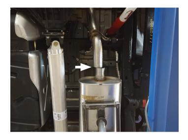
6. Disassemble passenger side tailpipe wire hangers (x2) from isolators. Remove bolt and mount near outlet then remove assembly from vehicle. Retain bolt and mount for later use.
