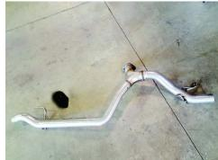
Loosen factory clamp from catalytic converter connection to disconnect inlet pipe, disassemble wire hanger from isolator then remove muffler assembly completely from vehicle.
