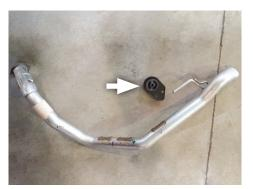
5. Cut tailpipes just behind factory muffler.
