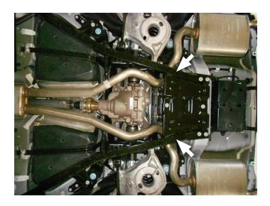
4. Measure and mark 2½" from beginning of straight section on exhaust pipes (x2) as shown. Support then cut pipes at marks. Unbolt hanger mounts and remove tailpipes from vehicle.
