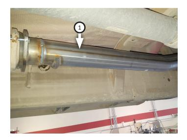
8. Place extension pipe hanger (8) onto extension pipe (2) then connect it to inlet pipe. Connect hanger to factory isolator then tighten clamp just enough to allow for adjustment.
