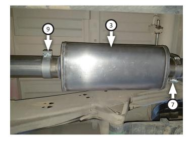
10. Route **front tailpipe (4)** over axle and connect it to muffler. Make sure its oriented properly then tighten front clamp just enough to allow for adjustment.
