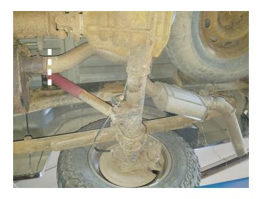
4. Support muffler and disassemble wire hangers from isolators. Loosen ring clamp, disconnect inlet pipe then remove exhaust system.
