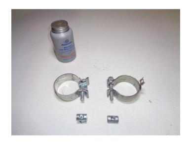
6. Place **clamp (2)** onto **muffler assembly (1)** lining notch up to tab then connect it to inlet pipe and insert wire hangers into isolators then tighten clamp.
