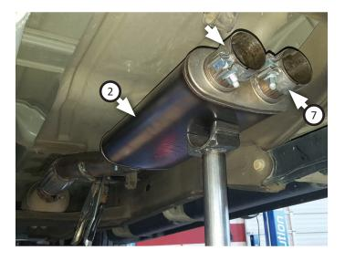
9. Route **left (3)** and **right (4)** pipes over axle then connect them to muffler. Insert their wire hangers into isolators then tighten clamps just enough to allow for adjustment.
