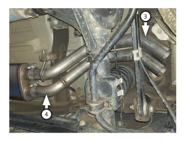
10. Place (x2) **clamps (7)** onto **exit pipe (5)** then connect it to over axle pipes. Insert wire hanger into rubber hanger then tighten clamps just enough to allow for later adjustment.
