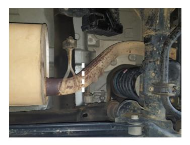
Support muffler and disassemble wire hangers from isolators. Remove and retain (release tab to remove) ball clamp, disconnect inlet pipe at cat. converter and remove muffler section from vehicle.
