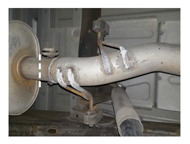
4. Support muffler and disassemble wire hangers from isolators. Loosen ball clamp, disconnect pipe at catalytic converter and remove exhaust system. Release tab to remove clamp from pipe and retain it for later use.
