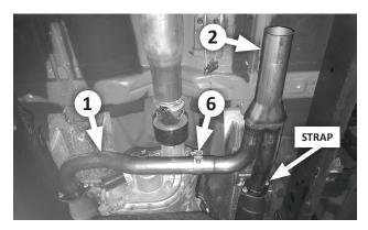
7. Slip a 2-1/2" clamp (6) over the head pipe assembly (2), slip the head pipe assembly over the left head pipe (1), then attach the pipes to the catalytic converter flanges using the stock gaskets and fasteners. (Reattach the bonding strap if applicable.) Verify 3" of insertion, and snug the clamp slightly (just enough to allow final adjustment later).
