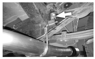
12. Adjust the tailpipe assembly so the pipes clear the frame and the tips are at the desired distance from the body. Lay the rear frame hanger flat against the inside of the truck's frame, and mark the hole locations. Move the bracket aside, drill 1/4" holes at the marks, and fasten the bracket to the frame with the two thread-cutting screws (12).
