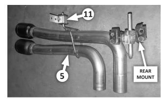
10. Install rear frame hanger (11) on the tailpipe assembly's(5) thin hanger rod. Install the muffler's rear isolator mount (removed at Step 5) on the thick hanger rod.
