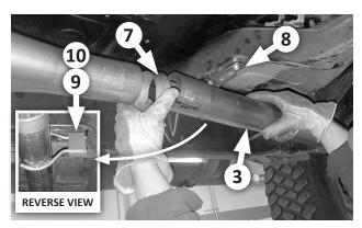
8. Install front hanger bracket (8) with 2 stock screws. Slip a 3" clamp (7) over extension pipe (3), slip the extension pipe over the headpipe, then install rubber hanger (9) on the bracket and pipe's hanger rods. Verify 3" of insertion, and snug the clamp slightly. Install the two 7/16" hanger keepers (10) on the hanger rods.
