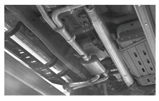
**13.** Adjust all components to give 1/2" to 3/4" clearance (about a finger's width) around them, and allowing for suspension travel and vibration. When you are satisfied with the system's clearance and fit, tighten all clamps.
