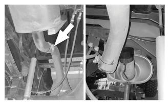
Loosen the clamp behind the muffler, and separate the tailpipe from the muffler.
