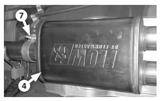
9. Slip the other 3" clamp (7) over the muffler's (4) inlet. Then install the muffler on the extension pipe and support it with a stand. Verify 2" of insertion, and snug the clamp.
