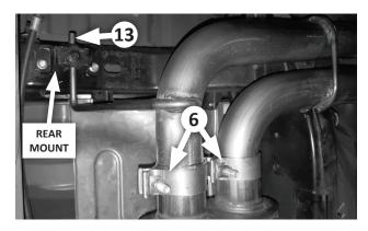
11. Slip two 2-1/2" clamps (6) over the muffler outlets. Insert both tailpipes in the muffler, and fasten the isolator mount to the frame using the stock screws. Verify 2" of insertion, and snug the clamps. Install the 1/2" hanger keeper (13) on the hanger rod.
