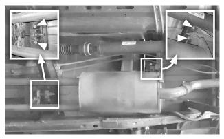
5. Remove and retain the 2 screws from both the front and the rear isolator mounts. Remove the assembled headpipes, muffler, and mounts from the vehicle.
