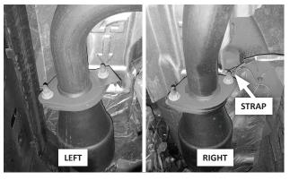
4. Remove and retain the fasteners and gaskets from the 2 flanges where the head pipes meet the catalytic converters. (One of the fasteners may secure a bonding strap.)
