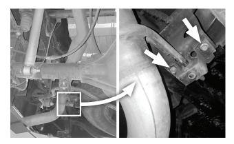
Remove the 2 screws from the tailpipe's isolator mount.
