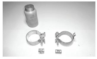
Before installing any clamps, remove their nuts, apply antiseize compound to the bolt threads, and re-install the nuts.
