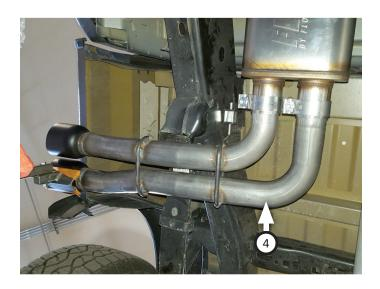
13. Verify system is properly positioned, then insert bracket (11) onto exit pipe assembly. Set bracket against vehicle frame and mark holes. Remove bracket, drill holes then fasten bracket in place with bolts (removed step 10).
