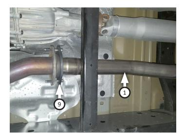
9. If applicable, place clamp (7) onto extension (2) then connect it to inlet pipe. Tighten clamp just enough to allow for adjustment.
