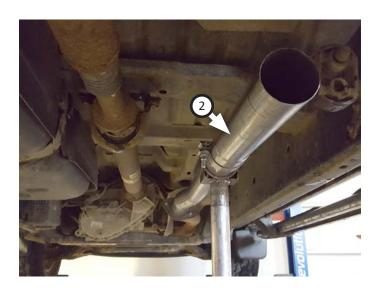
10. Remove muffler hanger mount, slide it onto muffler (3) and place clamp (5) onto muffler. Connect muffler to inlet/extension then fasten hanger mount into place on frame. Tighten clamp just enough to hold parts.
