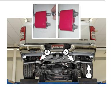
17. Recommended: apply one inch tack weld to all slip-fit connections then apply high temperature paint over each weld to prevent rust and premature corrosion.
