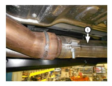
8. Place **clamp (14)** onto **extension pipe (2 or 3)** then connect it to inlet pipe. Connect wire hangers to isolators then tighten clamp just enough to allow for adjustment.
