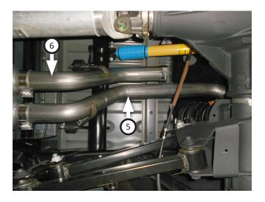
12. Place **clamp (15)** on **left rear tailpipe (7)** then connect it to left front tailpipe at slip-fit connection over rear axle. Place rear hanger into rubber hanger then tighten clamp just enough to allow for adjustment.
