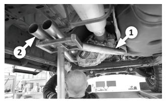
7. Attach left (2) and right (1) inlet pipes to factory exhaust with the 2 stock gaskets, and 4 screws and springs, ensuring that both pipes are oriented properly.
