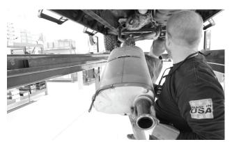
5. Disengage muffler rods from rubber isolaters (3 places), and remove muffler and pipe assembly from vehicle. Remove and retain 2 flange gaskets. Retract the spare tire to its stowed position.
