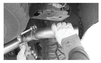
**15.** Slip a clamp (11) over each side exit pipe (9), and install each exit pipe on its tailpipe. Align each exit pipe as desired, verify 3" of insertion, and snug each clamp slightly.
