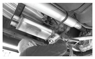
11. Slip two clamps (11) over the muffler's (3) inlets (the end with the hanger rods). Install the hanger rods in the rubber isolators, then install the muffler on the inlet pipes. Verify 2" of insertion, and snug the clamps slightly.
