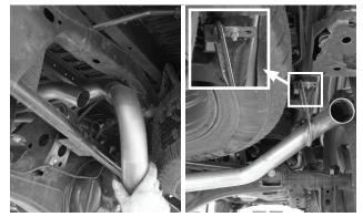
13. Slip a clamp (11) over the right over-axle pipe. Install the universal bracket (12) on the right tailpipe's (6) hanger rod, with the flat pointing outboard and facing up toward the frame. Slip the tailpipe over the over-axle pipe. Then fasten the bracket to the frame with the bolt (13) and a flat washer (15) against the frame, and the other flat washer (15), the lock washer (16), and the nut (14) against the bracket. Verify 3" of insertion, and snug the clamp slightly.
