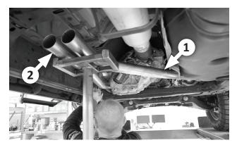
**7.** Attach left and right inlet pipes (2 and 1) to factory exhaust with the 2 stock gaskets, and 4 screws and springs, ensuring that both pipes are oriented properly.
