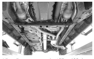
**14.** Adjust all components to give 1/2" to 3/4" clearance (about a finger's width) around them, and allowing for suspension travel and vibration. When you are satisfied with the system's clearance and fit, tighten all clamps.
