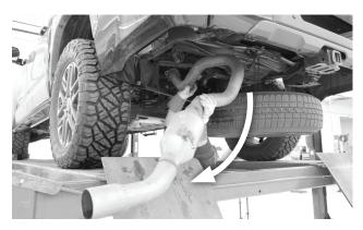
Lower the spare tire for clearance, and remove the tailpipe from the vehicle.
