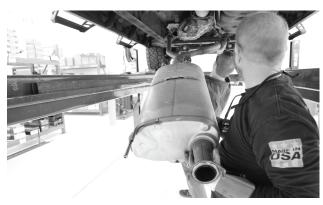
5. Disengage muffler rods from rubber isolaters (3 places), and remove muffler and pipe assembly from vehicle. Remove and retain 2 flange gaskets. Retract the spare tire to its stowed position.
