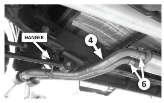
**13.** Slip clamps (6) over the muffler's outlets. Move the tailpipe assembly (4) into place, insert its hanger rod into the frame hanger, and insert the pipes into the muffler. Verify 2" of insertion, and snug the clamps slightly.
