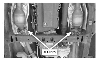
Remove and retain 4 screws and springs at the 2 catalytic converter flanges.
