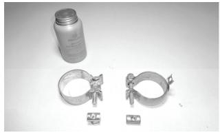
**6. Before installing clamps in the following steps,** remove their nuts, apply anti-seize compound to the bolt threads, and re-install the nuts.
