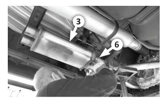
11. Slip two clamps (6) over the muffler's (3) inlets (the end with the hanger rods). Install the hanger rods in the rubber isolators, then install the muffler on the inlet pipes. Verify 2" of insertion, and snug the clamps slightly.
