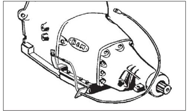
2. Install the B&M selector lever on the selector shaft with the supplied lock nut, and tighten the nut to 23 ft-lbs. Verify that the selector lever moves freely through all positions.
