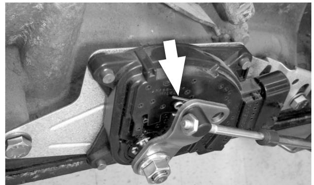
8. Secure the swivel to the selector lever with the cotter pin. Operate the shifter through all the gear positions, verifying that it operates correctly.
