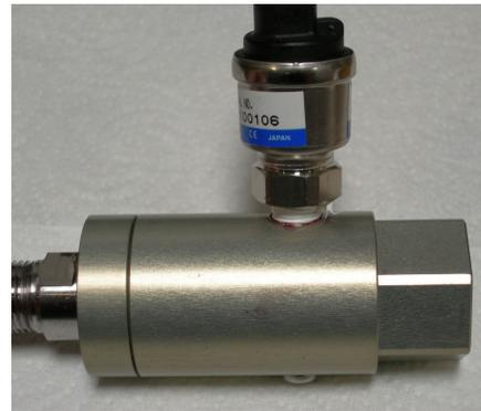
4. Remove bleed screw on load cell opposite of sensor port. Using a paper clip (or similar item) break air bubble that is formed by the fluid at this opening. Add extra fluid if needed.
