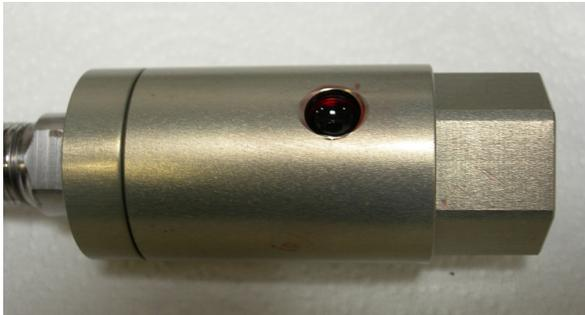
3. Carefully install sensor into load cell sensor port trying to minimize fluid loss during process.
