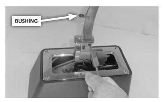
**6. Insert the bushing in the new stick,** then insert the stick in the shifter. Apply thread locking fluid to the 2 screws, then install and tighten the screws.
