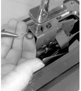
**3.** Place a fingertip under the trigger rod to catch the washer, then pull the hair pin with needle-nose pliers, and set the pin and washer aside.
