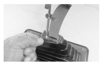
9. Gently work the rubber boot down over the stick and work the boot's lower groove onto the chrome cover. Then work the boot's upper groove onto the stick's lower flange. (The stick has 2 flanges, and the top flange will sit atop the boot.) **10. Run the jam nut all the way** down the stick's threads. Then apply thread locking fluid to the stick threads.
