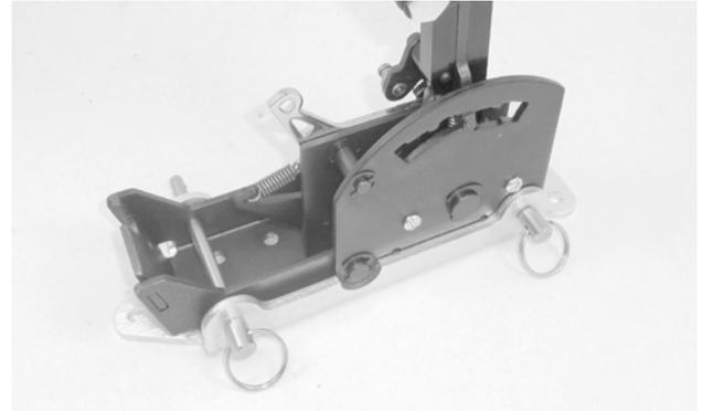
2. **Pin the shifter to the bracket** with the two quick release pins.
