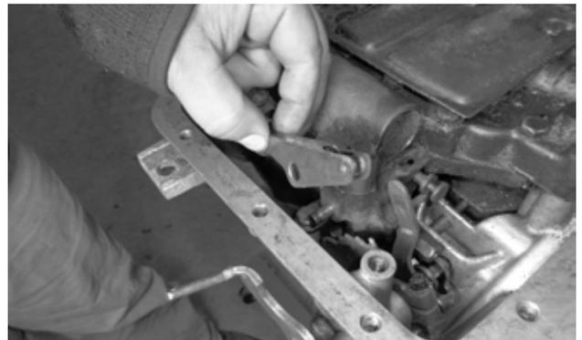
**14. Remove the detent roller by removing its E-clip.**
