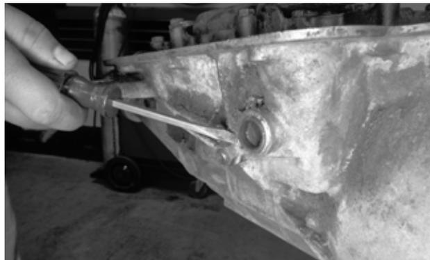
17. Inspect the selector shaft seal in the transmission case. Replace if required. Lubricate seal with a thin film of transmission fluid.
