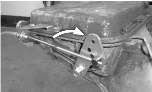
**30. With the swivel still in the selector lever, push the shifter all the way forward to the PARK position.** Verify that the swivel still slips freely in and out of the **B&M 1** hole in the selector lever. If not, adjust the swivel (and / or the cable housing nuts, if necessary), until it does.
