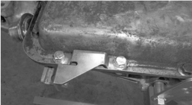
**26. Install the cable bracket** at the two rear holes, using the two **5/16-18 x 1" bolts** and **lock washers**. Tighten the pan bolts to 7-10 ft-lbs torque.
