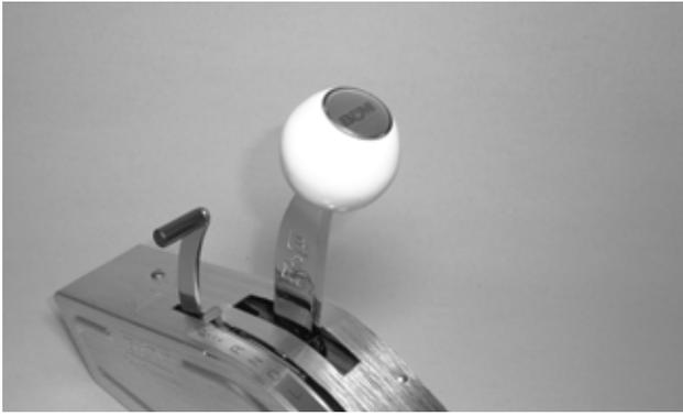
**37. Install the shifter knob:** Apply **medium strength thread locker** to the shifter threads.
