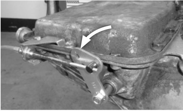
**29. Manually move the selector lever to the LOW (full-rear) position.** Ratchet the shifter handle to the LOW position (furthest back). Adjust the cable housing nuts until the swivel slides freely in and out of the **B&M 1** hole in the selector lever. Gradually tighten the nuts against the bracket, while continuing to check the fit of the swivel in the selector lever. When the swivel slips freely in and out of the selector lever, snug the jam nut.
