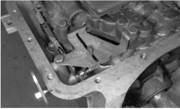
**24. Reinstall the manual valve guide plate** while ensuring that the selector lever pin remains engaged in the manual valve groove. Tighten the two bolts to 15 lb-ft torque. Verify that the selector lever travels back and forth freely and smoothly, with a positive click in each selector position.
