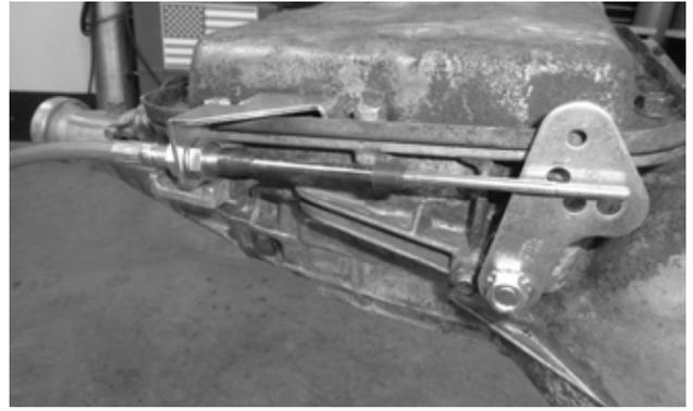
**27. Attach the shifter cable to the cable bracket:** First remove the small jam nut, two plastic dust boots, and one large nut and lock washer from the cable housing. Then insert the cable housing in the cable bracket, reinstall the lock washer and large nut on the cable (loosely, to allow room for adjustment), and reinstall the two dust boots.
