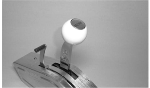
63. Install the shifter knob: Apply medium strength thread locker to the shifter threads.
