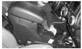
Remove the console base to access the stock shift cable. Refer to your vehicle's service manual for detailed instructions.
