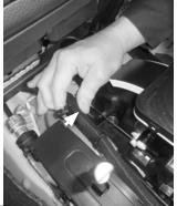
**5. Detach the wire loom clamp** from the front passenger-side of the shifter base.
