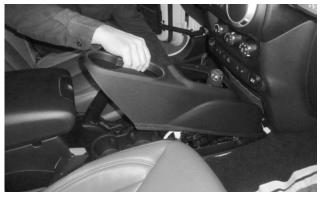
**41. Reinstall the center console** according to your vehicle's service manual.
