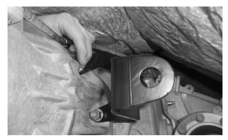
**13. Install the B&M transmission bracket [item 1].** Do not reinstall the wire loom bracket, as the stud is too short. (If necessary, use a cable-tie to secure the wire loom.)
