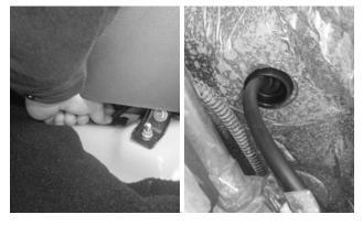
32. Work the floor grommet into the hole in the floor pan.
