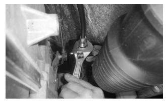
**37.** After verifying adjustment, tighten the large jam nuts at the transmission bracket.
