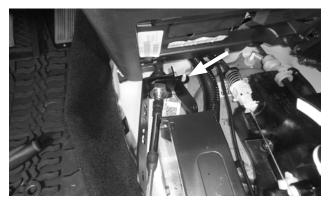
21. Slip the large bracket over the shifter base mount stud (nut removed at Step 18).
