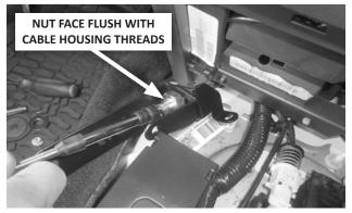
**20. Install the jam nut only (not the washer) on the cable housing,** and run it down until its face is flush with the rear thread.
