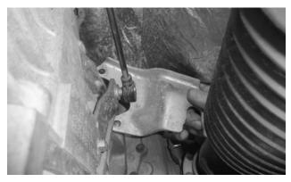
12. Remove the 2 nuts, the wire loom bracket, and the transmission bracket.
