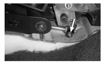
**31. Install e-clip [9] on the shift lever pin,** then tighten the jam nut.
