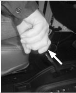
Remove the transfer case shift knob by grasping it firmly and pulling it off the lever.
