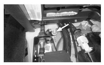
**24.** Hand-start the shifter base nut on its stud (over the large bracket).
