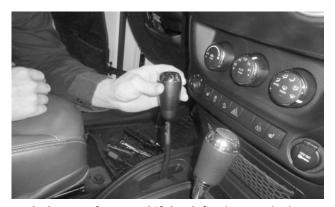
42. Push the transfer case shift knob firmly onto the lever.
