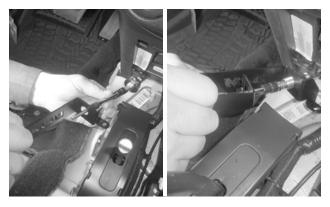
**19. Slip the large shifter bracket [2]** over the cable end, followed by the small shifter bracket [4].
