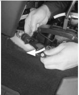
6. Carefully pry the cable out of the left side of the shifter base.
