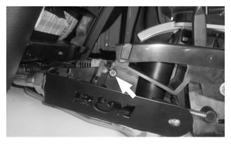
**25.** Hand-start screw [10] and nut [11] through the shifter and small bracket (screw head to the left, nut to the right).
