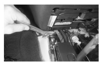
**29. Tighten the front jam nut** (closest to the dash) against the two shifter brackets and rear jam nut.
