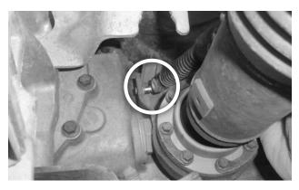
**10.** With a flat-tip screwdriver, pry the cable end off the pin on the range lever. Finish removing the cable from the floor pan hole and the vehicle.
