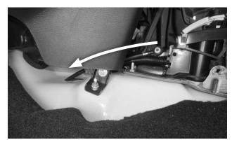
**8. Push the cable partially under the dash pedestal** and down through the floor pan.
