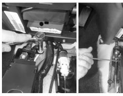
**27. Tighten the shifter base nut** (installed at **Step 24**) and the small bracket screw and nut (installed at **Step 25**).
