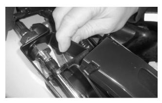
**23.** Work the small bracket to the right side of the shifter (where the wire loom was located).
