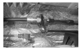
**33.** Install a jam nut and washer on the cable housing, feed the cable through the transmission bracket, then run the second washer and nut down finger-tight against bracket. Reinstall large dust boot over its joint.
