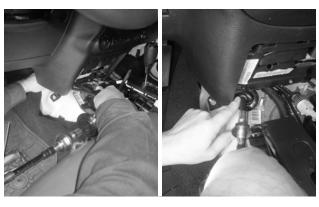
**16.** Feed the end of the cable without the jam nuts and washers down through the hole in the floor pan.
