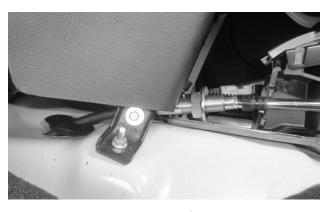
**17. Stop when the threaded section of the cable housing** reaches the dash pedestal. Remove (and retain) one jam nut from the cable housing, and remove (and discard) one washer.
