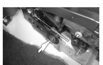
**26.** Temporarily install and tighten the stock console base screw and washer, securing the large shifter bracket to the shifter base.
