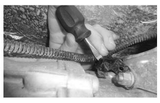
**11.** At the top of the transmission, disconnect the wire loom from its bracket.
