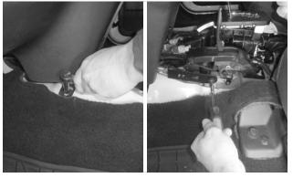
**39.** Tighten the pedestal bracket nut (loosened at Step 7). Then remove the console base screw and washer (temporarily installed at Step 26).
