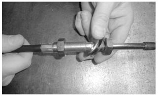
**14.** At one end of the cable [6], pull the large dust boot off its joint, then remove and set aside both jam nuts and washers.
