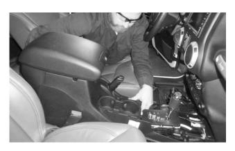
**40. Reinstall the console base** according to your vehicle's service manual.
