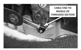
**30.** Install the jam nut [8] and the shifter cable end [3], locating the cable end in the middle of the threaded section. Then slip the cable end over the shifter pin.
