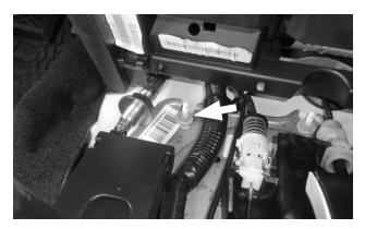
18. Remove the nut at the front left corner of the shifter base.
