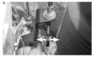
**35.** Verify that the shifter handle is in the "2H" position (fully forward), and that the range lever is moved fully forward. Then adjust the transfer case cable end as required, until it moves freely on and off of the pin on the range lever. Then finger-tighten the jam nut.
