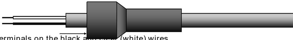
**Step 6:** Crimp the terminals on the black and clear (white) wires.
