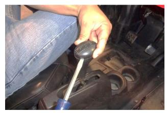
Turn off your vehicle's ignition and set the parking brake. Carefully remove the stock shifter handle cap with a flat tip screwdriver or plastic trim tool.
