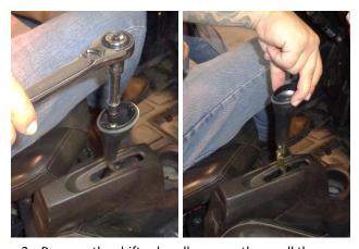
2. Remove the shifter handle screw, then pull the handle off the shifter lever.
