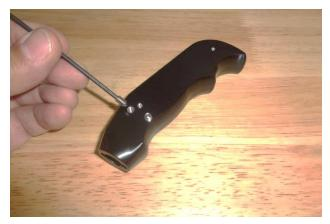
3. Thread the 4 set screws (Item 5) about 2-3 turns into the shifter handle body (1). (Two screws each side.)
