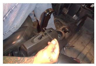
5. Tighten all 4 set screws to secure the shifter handle to the shifter lever.
