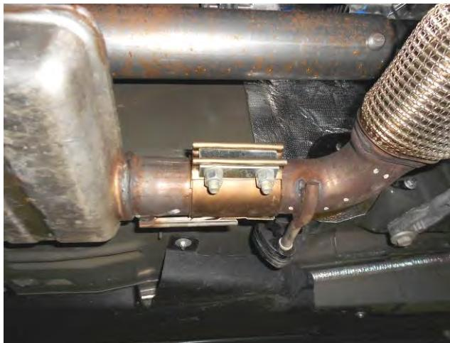
4) Using a 15mm wrench, loosen the two bolts at the clamp connection in the center of the vehicle. Use a small screwdriver to lift the clip and with the help of an assistant, carefully lower the stands at the rear of the resonator and slide the system toward the rear and off of the front pipe. Lower the resonator from the vehicle. The clamp should remain on the factory front pipe as it will be re-used with the new Flowmaster system.
