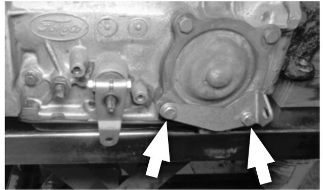
A. C4 / C5 transmissions: Install the cable bracket at the two lower servo cover bolt holes, using the two 5/16-18 x 1" bolts, spacers, and lock washers. Tighten the bolts to 12-13 ft-lbs torque.
