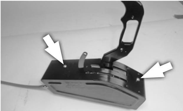
**E. Release the stick, allowing it to return to its centered position. Then fasten the cover to the shifter with the two 10-32 screws.**
