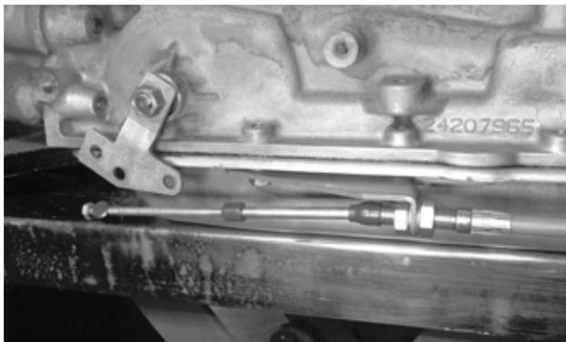
**48. Attach the shifter cable to the cable bracket:** First remove the small jam nut, two plastic dust boots, and one large nut and lock washer from the cable housing. Then insert the cable housing in the cable bracket, reinstall the lock washer and large nut on the cable (loosely, to allow room for adjustment), and reinstall the two dust boots.
