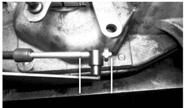
16. Thread the swivel onto the cable to about the middle of the threaded section, then reinstall (but do not tighten) the jam nut.
