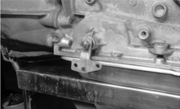
45. **Install the B&M selector lever** using the stock selector lever nut, and tighten the nut to 23 ft-lbs torque. The lever should travel smoothly back and forth, with a positive “click” in each position.
