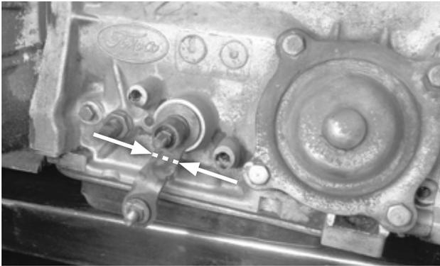
29. If the stock selector lever points generally downward, cut it off at the inboard bend, in order to allow the B&M lever to be positioned correctly.
