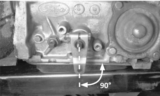
30. Install the B&M selector lever using the 1/4-20 x 1-1/2" bolt, lock washer and nut. With the selector shaft in NEUTRAL (the second click back from PARK, which is full-forward), align the selector lever perpendicular to the oil pan split-line, then tighten the fasteners.
