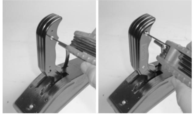
**63. Assemble the shifter grip:** First install the left- and right-side spacers on the shifter handle, using the two 6-32 x 3/4" flat head screws. Then install the two side plates, using four 6-32 x 3/8" flat head screws.
