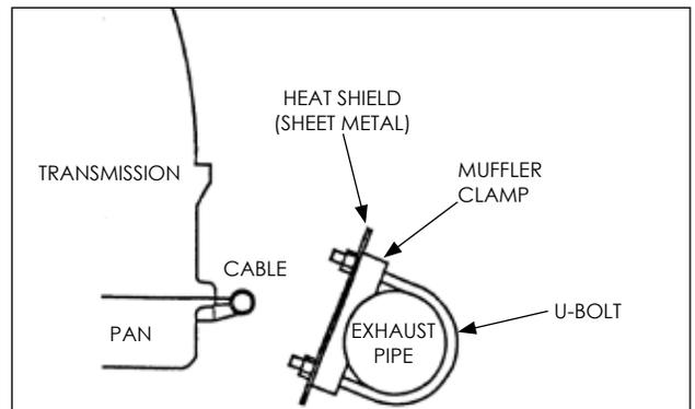
**CAUTION:** Heat will severely damage the shift cable, causing the housing to melt or become brittle. If the cable must be routed near exhaust system components, fabricate a heat shield. **Do not wrap the cable, as this retains heat.**
