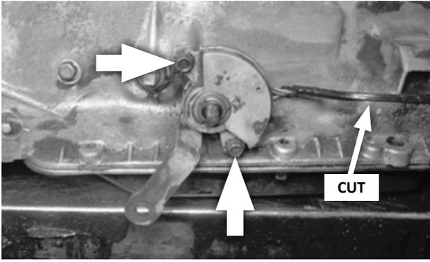
28. If your transmission is equipped with a Neutral Safety / Backup Light switch: Remove the two mount bolts and slide the switch off the selector shaft. Cut the wiring harness between the switch and its connector, and discard the switch. (The wires from the connector will be routed to the B&M switches later.)
