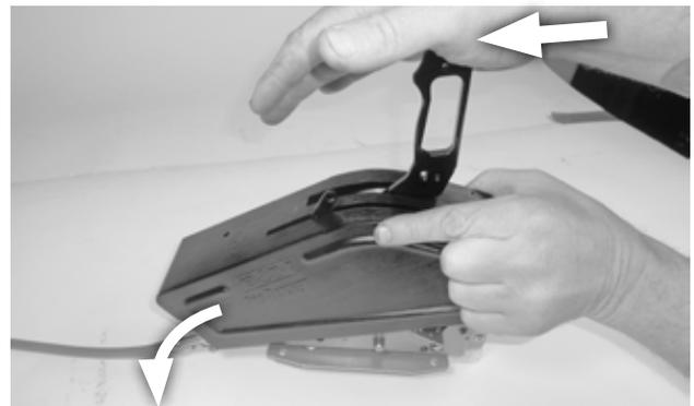
**C. Push the stick forward and hold it there,** lower the front of the cover over the front of the shifter, and **continue to hold the stick forward.**
