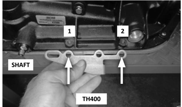
46. **Determine which holes on the cable bracket will be used:** Remove the two oil pan bolts to the rear of the selector shaft. Determine which bracket holes will be used on your transmission.
