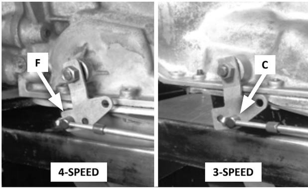
51. Adjust the cable housing nuts until the swivel slides freely in and out of the correct hole in the selector lever (hole F for 4-speeds; hole C for 3-speeds). Gradually tighten the nuts against the bracket, while continuing to check the fit of the swivel in the selector lever.
