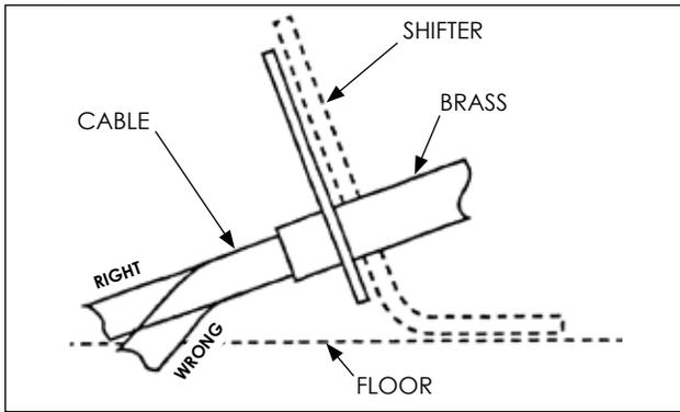
**CAUTION:** Do not kink the cable anywhere along its length, or it will lock up. The cable should be kept straight for at least 2" after it leaves the brass at each end.
