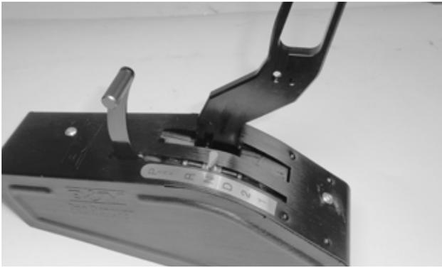
**62. Install the red aluminum handle on the left side of the reverse lockout lever using the 8-32 button head screw. Screw the red shifter position indicator pointer through the slot into the indicator arm. Use a medium strength thread locker to prevent the pointer from backing out in use. Select the shifter position indicator decal that is applicable to your transmission's valve body (see "Operation" NOTE), and affix it to the left of the pointer.**
