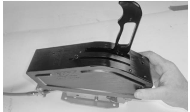
**B. Verify the shifter mechanism is free of any debris and hardware.** Lower the cover over the tips of the stick and the reverse lockout lever.
