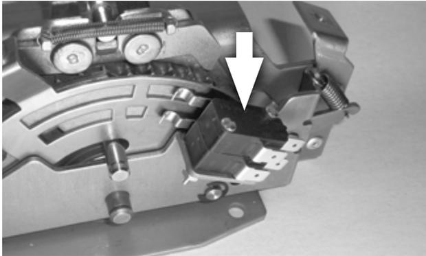
**8. Install the two switches on the shifter mechanism** as shown, using the two **#4-40 × 1-1/4" screws, lock washers and nuts.**
