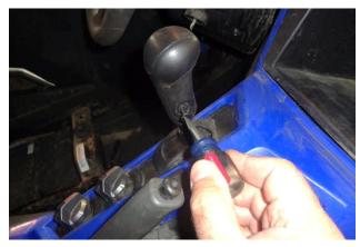
1. <u>Turn off your vehicle's ignition and set the</u> <u>parking brake</u>. Remove the fastener from the right side of the shifter handle.
