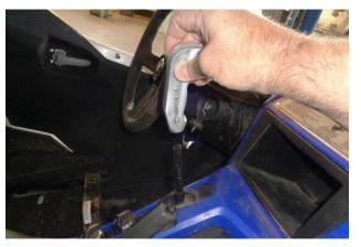
4. Slide the shifter handle body all the way onto the shifter lever.
