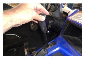
2. Pull the shifter handle off the shifter lever.
