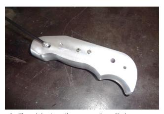
3. Thread the 4 small set screws (Item 5) about halfway into the shifter handle body (1) (two screws each side). Thread the large set screw (4) about halfway into the right side of the shifter handle body.
