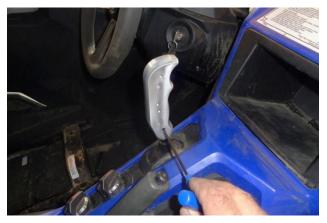
5. Tighten all 5 set screws to secure the shifter handle to the shifter lever.
