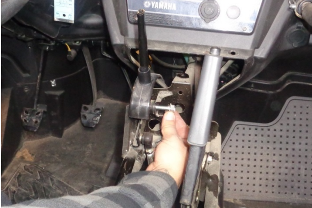
19. Remove the shift lever pivot nut and bolt, and retain them for use at Step 25.
