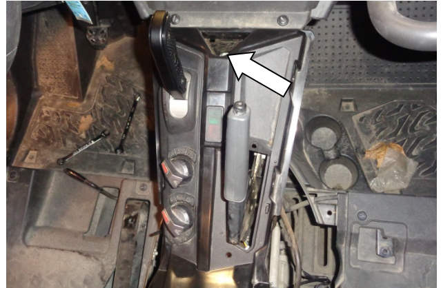
32. Reinstall the bolt at the front of the switch panel.
