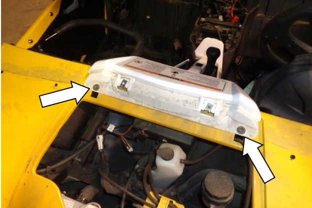
7. Remove the two screws at the front end of the front console cover.
