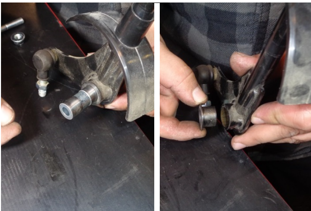
21. Remove the steel bushing from the shift lever, then remove the two plastic sleeves. Retain sleeves and bushing for use at Steps 23 and 24.
