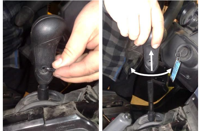
16. Carefully pry the plastic pin from the side of the shifter knob, then pull the knob up off the shift lever while twisting it side-to-side.
