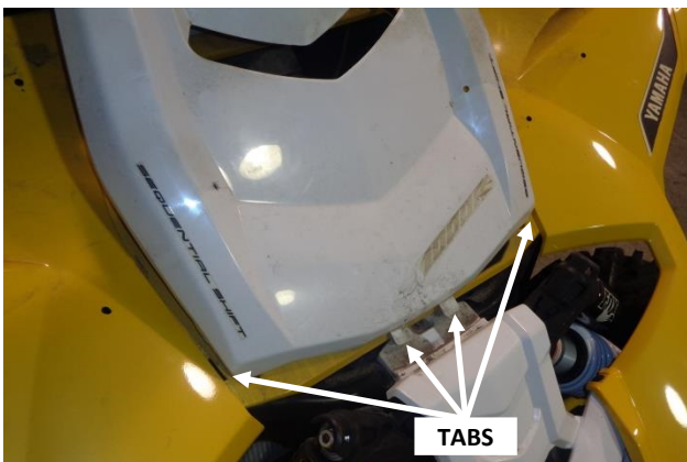
37. Insert the four tabs at the front of the service cover into their respective slots and lay the cover in place.
