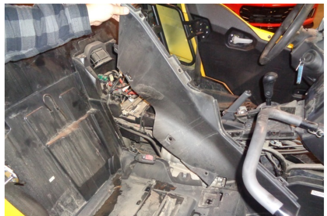
12. Carefully remove the right console side cover.
