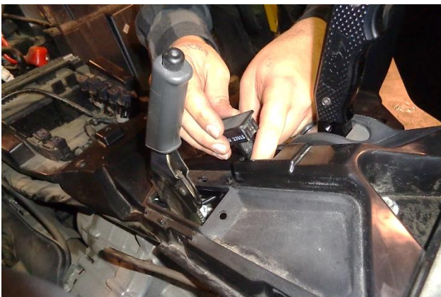
31. Reconnect the seat belt safety light to its electrical plug, then press the light back into the switch panel.
