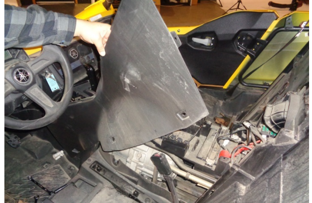
10. Carefully remove the left console side cover.
