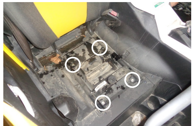
40. Reinstall the seat backs, fastening each one to the vehicle with its four bolts.
