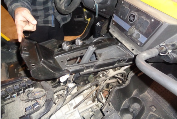
29. Place the switch panel over the shifter and parking brake handles.
