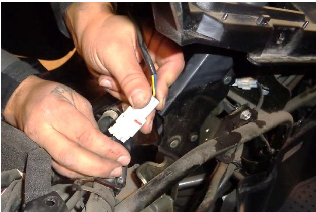
30. Reconnect the two rotary switch lead plugs. NOTE: The plugs have different shapes to prevent misconnection.
