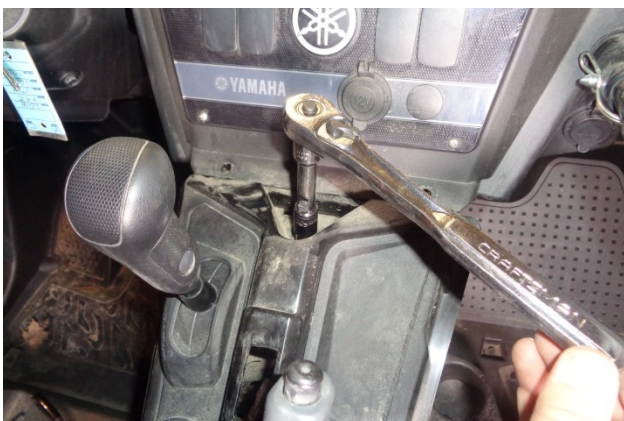
15. Remove the bolt at the front end of the switch panel.
