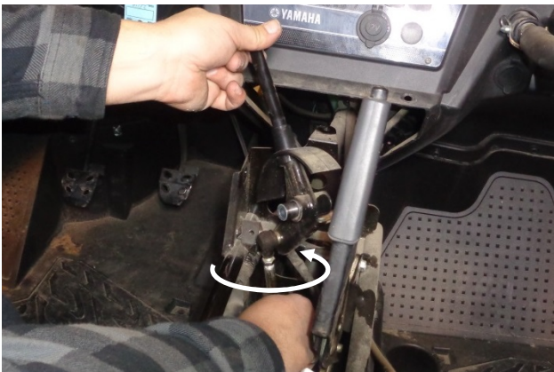
20. Spin the shift lever counter-clockwise to remove it from the end of the shift rod.
