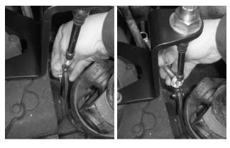
**14. Attach the clevis to the range lever** with the clevis pin and cotter pin, then tighten the jam nut against the clevis.
