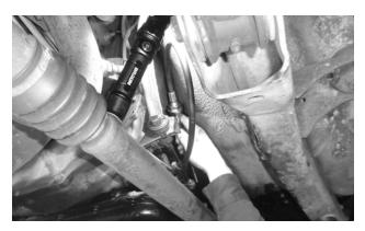
15. Install 1 washer (removed at Step 10) on the cable housing. Then route the cable forward along the transmission and back through the floor pan bracket, toward the shift lever. Avoid any obstacles (such as wiring harnesses, fluid lines, the transmission shift mechanism, etc.).
