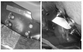
**11. Install the floor bracket** using 4 bolts [6] and washers [8]. Tighten the bolts until 5-6 threads protrude through the well nut.
