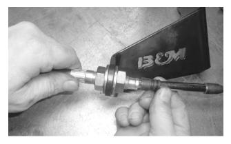
8. Assemble the cable [4] and transmission bracket [1] as shown. Pull the large dust boot off the joint to allow removal and installation of the jam nut. Situate the bracket in the middle of the threaded section, and run the nuts finger tight against it. Then push the dust boot back over its joint.
