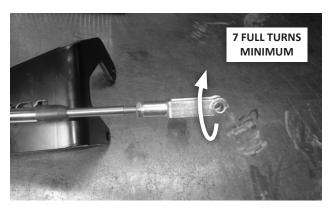
9. Install the jam nut [9] on the cable end. Then install the clevis [5] a minimum of 7 full turns onto the cable, and run the jam nut up against the clevis finger tight.
