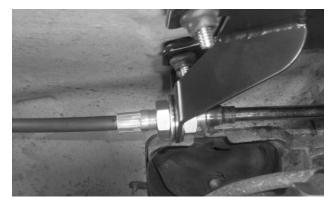
16. Install the second washer and jam nut on the cable housing. Center the bracket in the middle of the threaded section, run the nuts finger tight against it, and push the dust boot back over its joint.
