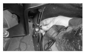
**13. Install the bushing [3] in the range lever.** A dab of grease or RTV will keep it in place until the clevis is connected.
