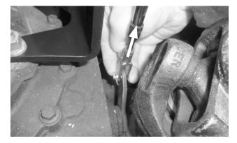
**18. Before adjusting the cable,** verify that the shifter handle is in the "2H" position (fully lowered), and that the range lever is moved fully-forward.
