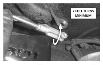
17. Install the jam nut [9], then install the clevis only [5] (no clevis pin or cotter pin), turning it a minimum of 7 full turns onto the cable.
