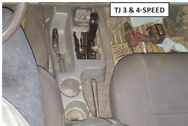
46. Re-install lower console (removed step 8) into center while routing wires to transfer case shifter.
