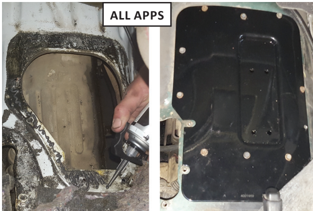
29. Install base plate using gasket. For more waterproofing, use silicone.
