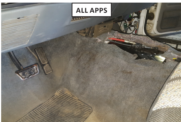
30. Choose rubber grommet (30,38) that is the closest size to your factory grommet. Remove hardware from threaded end of cable (4) and install grommet.
