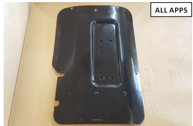
28. Using stamped indents for reference, drill holes matching your factory base. Choose hole size based on your preferred fasteners. For more secure mounting, use rivets over factory hardware.
